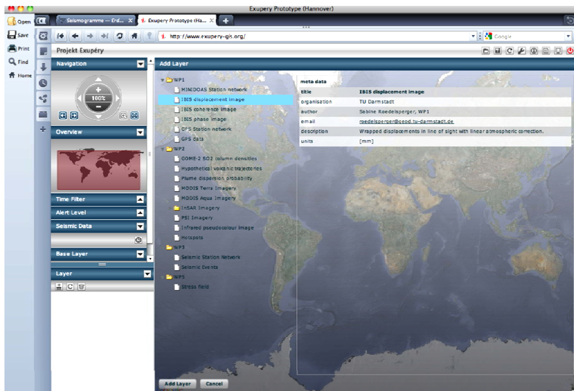
Fig. 13.45 Snapshot of the Exupery GIS. The browser-based application can include ground-based parameter sets and data as well as display 2D InSAR sections and 3D models.
