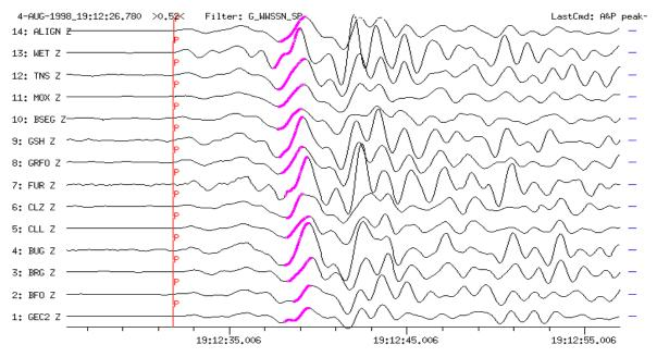
**Figure 13b:** After short-period filtering (WWSSN-SP simulation) the coherency of the different station-waveforms is bad. The maximum double P-amplitudes used for mb-estimation are emphasized. Because of the variability of station amplitudes within the network individual mb-values vary between 6.0 for BFO and GEC2 and 6.7 for other stations.
