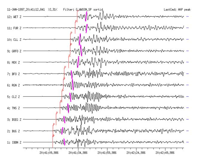
**Figure 12b** Records at the same stations as in Figure 12a, however after application of a short-period WWSSN-LP simulation filter. This is necessary for amplitude and period measurements required for standardized mb body-wave magnitude determinations. Maximum double-amplitudes (2A) and half-periods (T/2) are marked for the first wave group. Later onsets may belong to secondary or depth phases.
