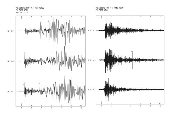
**Figure 1e** Low-pass (left) and high-frequency band-pass filtered (0.5-5 Hz) seismograms of the same earthquake recorded at station KIV (Kislovodsk; Russia) at the distance  $D = 15.2^{\circ}$ . The horizontal components N and E have been rotated into the R and T direction. No long-period waves are visible in the high-frequency record (courtesy of Lars Ottemöller, 2002).
