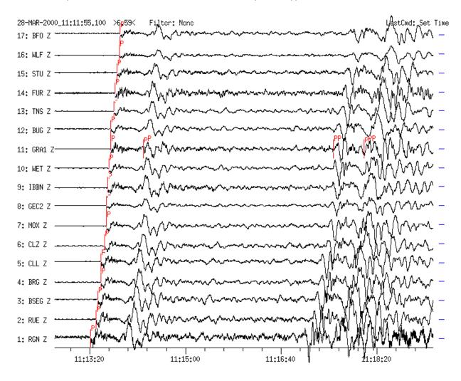
**Figure 15a** Broadband vertical-component seismograms recorded at 17 GRSN-, GRF- and GEOFON-stations. Traces are sorted according to increasing distance ( $D = 92.4^{\circ}$  to RGN and 99.1° BFO). The phases P, PP and the depth phases pP and pPP are recorded very well.
