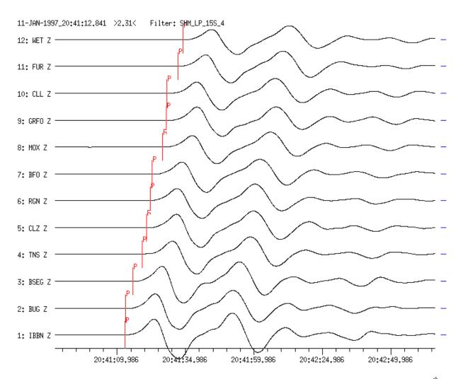
**Figure 12c** Records at the same stations as in Figure 12a, however after application of a  $4^{th}$ -order Butterworth low-pass filter (fc = 15 s). They show the long-period energy content of the earthquake with P-wave periods of about 20s! All long-period network traces are coherent. In this case the network can be used as an array.
