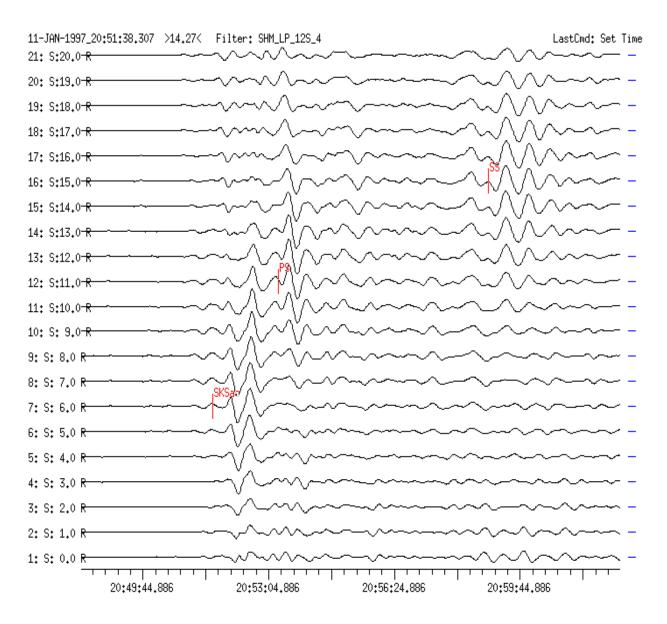
**Figure 12f** The identified phases from the radial-component vespagram are marked on slowness the respective slowness traces (SKSac on trace 7 with a slowness  $S = 6 \text{ s/}^{\circ}$ , PS on trace 12 with  $S = 11 \text{ s/}^{\circ}$  and SS on trace 16 with  $S = 15 \text{ s/}^{\circ}$ ).
