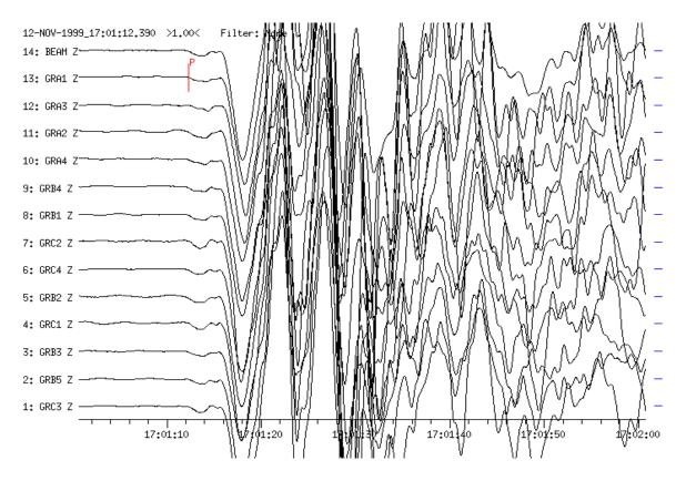
**Figure 2c** Broadband vertical-component seismogram with P-wave onsets recorded at all GRF-array stations. Traces are sorted according to increasing distance ( $D = 12.86^{\circ}$  from GRC3 and  $13.03^{\circ}$  from GRA1) and shifted in time according to a reference station (beamforming). All signal onsets are coherent. The weak first arrival of the P-wave onset is marked on the GRF-station GRA1.
