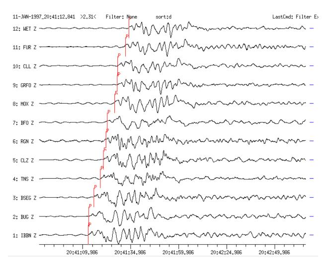
**Figure 12a** Broadband vertical-component seismograms recorded at 12 GRSN-stations are shown. Traces are sorted according to increasing distance of the stations ( $D = 87.7^{\circ}$  to IBBN and 92.1° to WET). P-wave onsets are marked.
