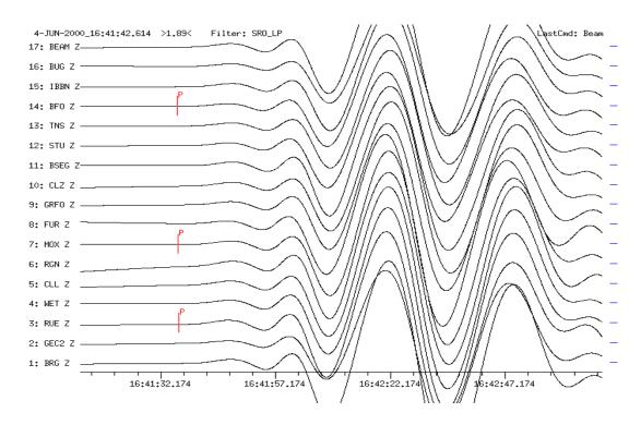
**Figure 14b** Seismograms of the same earthquake recorded at the same stations as in Figure 14a after applying a long-period filter (SRO-LP simulation). Note the very high signal coherence of the long-period P-waves with periods  $T \approx 25$  s. Also the amplitudes are comparable at all stations.
