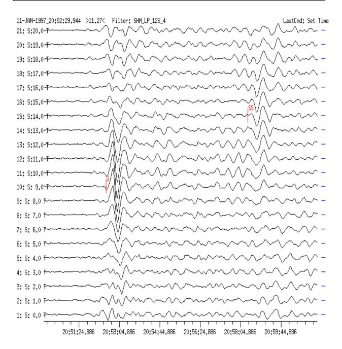
**Figure 12g** The identified phases from the transverse-component vespagram are marked on their respective slowness traces (S on trace 10 corresponding to a slowness  $S = 9 \text{ s/}^{\circ}$ , SS on trace 15 with  $S = 14 \text{ s/}^{\circ}$ ). Note, by comparing the identifications in Figs. 12e to 12g that the associated slowness values might somewhat differ because the maximum amplitudes vary only slightly when changing the slowness for about  $\pm 1 \text{ or } 2 \text{ s/}^{\circ}$ .
