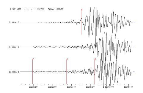
**Figure 1d** KIRNOS-filtered three-component seismogram from the GRF-array station GRA1 ( $D = 14.55^{\circ}$ ,  $BAZ = 138^{\circ}$ ). The horizontal components N and E have been rotated into the radial (R) and transverse (T) direction. The onsets of the body waves P and S and of the long-period surface waves LQ (Q) and LR (R) have been marked.
