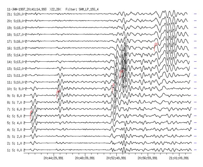
**Figure 12e** The identified phases from the vertical-component vespagram are marked on the respective slowness traces where they have their largest amplitudes (e.g. P on trace 6: belonging to a slowness  $S = 5 \text{ s/}^{\circ}$ , PP on trace 9 with  $S = 8 \text{ s/}^{\circ}$ , SP on trace 12 with  $S = 11 \text{ s/}^{\circ}$  and SS on trace 16 with  $S = 15 \text{ s/}^{\circ}$ ).
