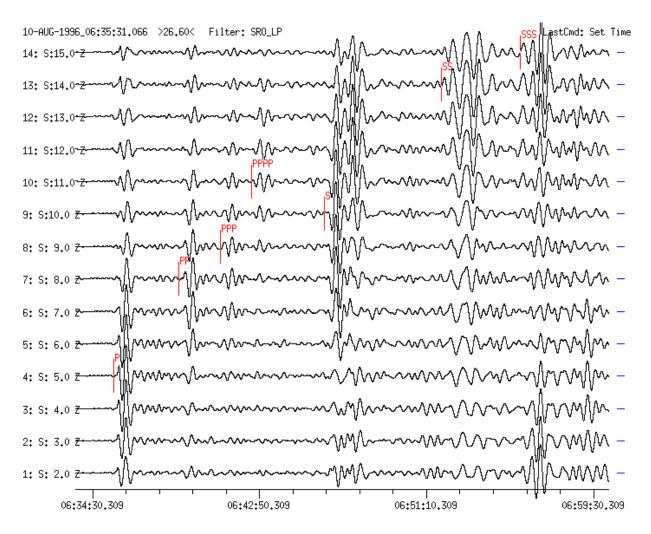
**Figure 11c** For better phase identification a <u>vespagram analysis</u> (see 9.7.7 in Chapter 9) of the long-period filtered traces was made. Identified phases have been marked on their respective slowness trace S (e.g., P on trace 4 with slowness S =  $5.0 \text{ s/}^{\circ}$  and PP on trace 7 with S =  $8.0 \text{ s/}^{\circ}$ ). In the vespagram traces the respective phases have the largest amplitudes at their proper slowness value.
