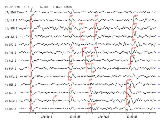
**Figure 6b** Stations and source parameter as in Figure 6a, however records of displacementproportional Kirnos-simulation. Phases P, PP and the depth phases sP, sPP are clearly visible on these records while the phase pP is recognizable only at GEC2.
