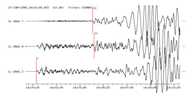
**Figure 3c** Three-component displacement-proportional KIRNOS-filtered seismogram recorded at the GRF-main-station GRA1 ( $D = 21.6^{\circ}$ ). The original N- and E- horizontal components have been rotated with R showing into the source direction. The time difference between the onsets SH (horizontal polarized S wave) and SV (vertical polarized S wave) is about 4 sec. The reason for this difference may be the anisotropy of upper mantle layers.
