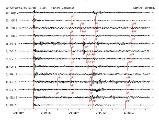
**Figure 6a** Short-period filtered seismogram (WWSSN-SP simulation) recorded at 12 GRSN, GRF(GRA1), GERESS and GEOFON stations. Traces are sorted according to distance ( $D = 42.4^{\circ}$  to BRG and 47.6° to WLF), shifted and aligned for P onsets. Note that the travel-time curves for PcP and PP intersect in this distance range. Depth phases pP and sP (see the marked theoretically expected arrival times) are not visible on this short-period filtered record.
