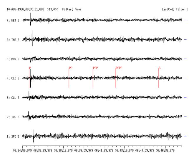
**Figure 11a** Broadband vertical-component seismograms of the Taiwan earthquake recorded at 7 GRSN-stations within the distance range  $D = 82.9^{\circ}$  and  $87.1^{\circ}$ . Only the P-wave onset is recognizable on the records. Secondary onsets such as surface reflections of the P and S wave (theoretical onset times marked on the CLZ trace) are not to be seen above the noise level.
