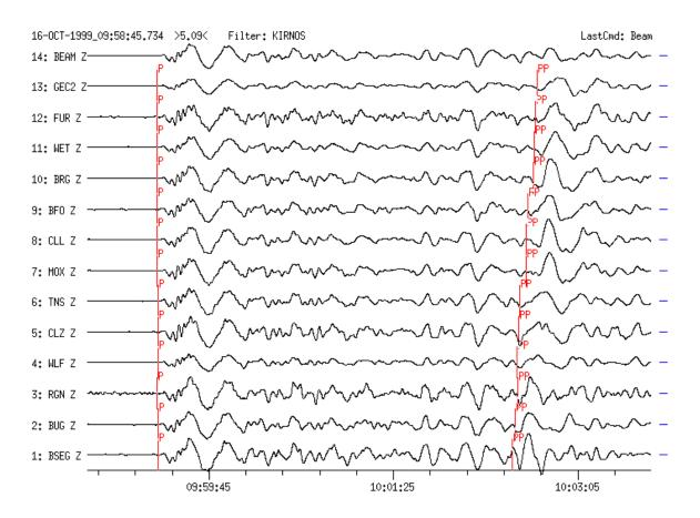
**Figure 9b** Broadband vertical-component seismograms recorded at 13 GRSN-stations. Traces are filtered (Kirnos-simulation), sorted according to increasing distance ( $80.1^{\circ}$  to BSEG and  $85.3^{\circ}$  to GEC2), shifted in time and aligned for P onsets. The used displacement proportional broad-band filter displays clearly the coherent part of the wave train from the network. As in Figure 9a, coherent phases appear ahead of PP that have slowness values as P.
