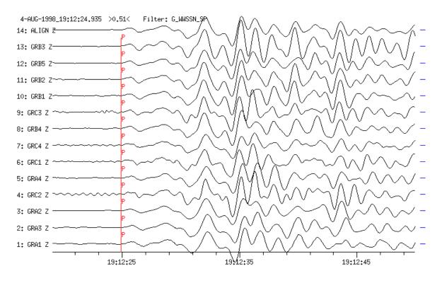
**Figure 13d** Even for the short-period filtered records of the GRF-array stations (WWSSN-SP simulation) the signal coherence is still good.
