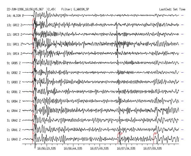
**Figure 7c** Short-period filtered seismograms recorded at the GRF-array. Traces are sorted according to increasing distance ( $D = 49.48^{\circ}$  to GRA3 and 50.33° to GRC2), shifted in time and aligned for P onsets. Phases P, PcP and PP have been marked. Because of the smaller spacing of the array-stations as compared with the GRSN stations, the decrease of the travel-time difference PcP-P is less obvious.
