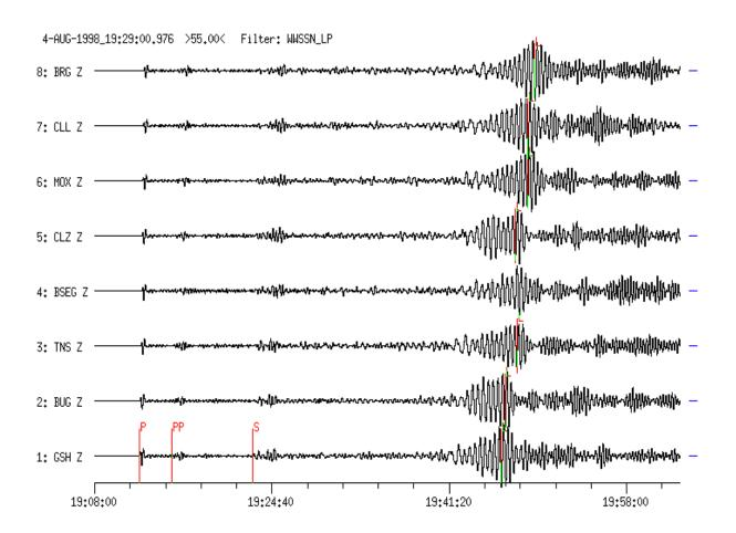
**Figure 13f** Long-period filtered (WWSSN-LP simulation) vertical-component records of the Ecuador earthquake at 8 GRSN stations within the distance range  $D = 88.4^{\circ}$  (GSH) to  $93.2^{\circ}$  (BRG). The variability of the maximum surface-wave amplitudes throughout the network is less than that of short-period body-wave amplitudes (compare with Figure 13b). Accordingly, Ms estimates from individual stations are more reliable than respective mb estimates.
