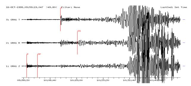
**Figure 9c** Broadband three-component seismogram recorded at GRA1 ( $D = 83.6^{\circ}$ ). The horizontal components are rotated into the R and T direction. Phases P, PP, S, SS and surface waves are displayed. Rayleigh waves recorded on radial and vertical components appear later than Love waves recorded on the transversal component only.
