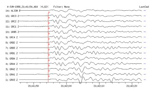
**Figure 4b** Broadband vertical-component seismograms recorded at the GRF-array stations. Traces are sorted according to increasing distance ( $D = 22.48^{\circ}$  to GRA3 and 23.27° to GRC3), shifted in time and aligned for better signal comparison. Because of the smaller aperture of the array as compared to the GRSN network signals are more similar. At the nearest stations (GRA3 up to GRA4) a second onset appears about 10 s after P.
