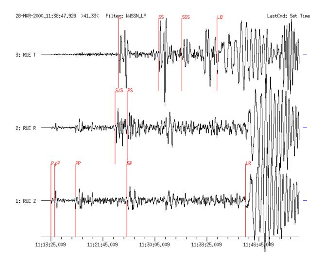
**Figure 15b** Long-period filtered (WWSSN-LP simulation) three-component seismogram of the Volcano Island earthquake recorded at station RUE near Berlin ( $D = 93.7^{\circ}$ ,  $BAZ = 45^{\circ}$ ). The horizontal components are rotated, with R in source direction. Phases P, pP, SP and the onset of the Rayleigh waves LR are marked on the vertical component, SKS and PS on the radial component and S, SS, SSS as well as the Love waves onset LQ on the transversal component, respectively.
