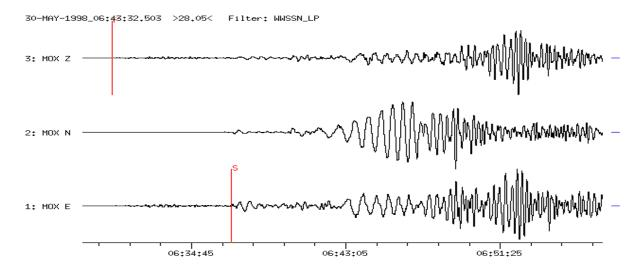
**Figure 5a** Three-component long-period seismogram (WWSSN-LP simulation filter) recorded at station MOX ( $D = 43.2^{\circ}$ ,  $BAZ = 85^{\circ}$ ) with P, S and dispersed surface waves. The nuclear explosion in Pakistan (see Figure 6.2) was recorded within the coda of this strong earthquake. As compared with the earthquake no surface waves has been recorded from the nuclear explosion.
