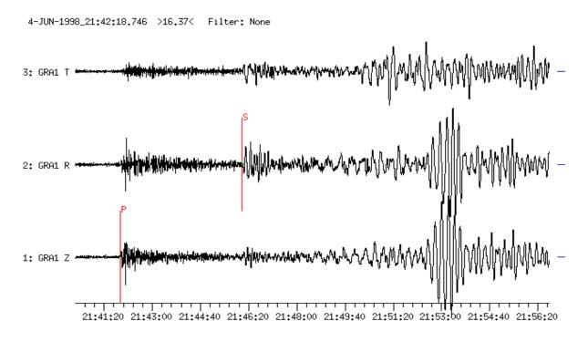
**Figure 4c** Simple three-component broadband seismogram at station GRA1 ( $D = 22.5^{\circ}$ ) with clear P, S and surface waves. Horizontal components have been rotated (ZRT) with R into source direction.
