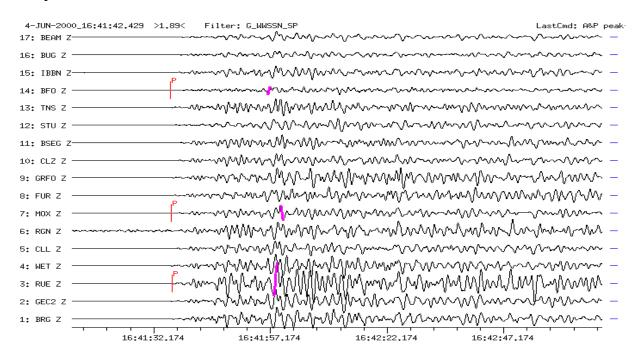
**Figure 14c** For mb estimates short-period records (WWSSN-SP simulation) have to be used to measure the maximum amplitudes with periods near 1 s. The respective filtered traces for the same earthquake and stations as in Figure 14a are shown. For three stations the P wave arrivals and their maximum double-amplitudes 2A have been marked. The latter differ by a factor of five for this event. This corresponds to a difference of 0.7 magnitude units!
