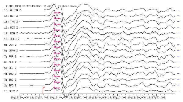
**Figure 13a** Broadband vertical-component seismograms recorded at 14 GRSN stations ( $D = 88.4^{\circ}$  to 93.2°). Traces are time-shifted and aligned. The different waveforms observed at different network stations are coherent in the long-period range.
