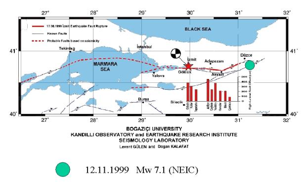
**Figure 2a** The Düzce earthquake of November 12, 1999 occurred about 110 km east of the earlier Izmit earthquake of August 17, 1999. The map shows the epicenter regions of both earthquakes together with one moment-tensor solution (for the Izmit event) and the right lateral surface displacement values (in cm) observed after the first shock.
