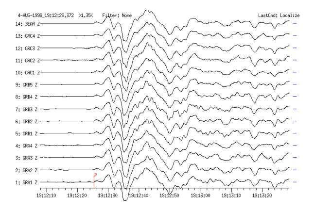
**Figure 13c** Broadband records of the vertical-components at 13 GRF-array stations (D =  $91.5^{\circ}$  to  $91.7^{\circ}$ ). Because of the much smaller aperture of the array as compared to the GRSN the signal coherence is good for all array-traces.
