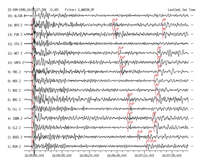
**Figure 7b** The same records as in Figure 7a, however, traces have been time-shifted and aligned for the P onsets. This figure shows more clearly the decreasing travel-time difference (PcP - P) with increasing distance from the epicenter.
