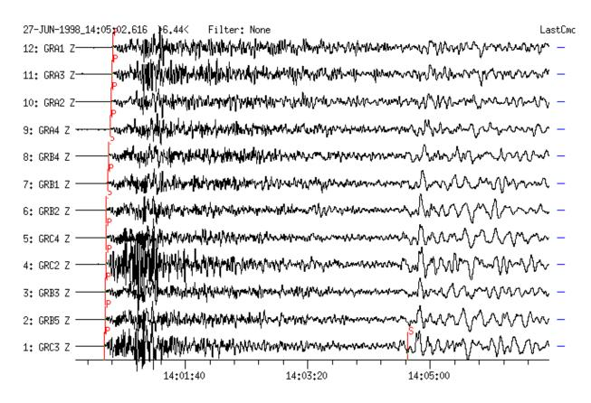
**Figure 3b** Broadband seismogram with P- and S-wave onsets recorded at 12 GRF-array stations. Traces are sorted according to increasing distance. P and S waves on the individual traces are influenced by upper mantle discontinuities and signals are also not coherent.
