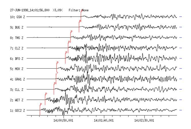
**Figure 3a** Broadband seismograms with high time resolution showing the complex P-wave groups. Records were made on vertical components of 10 GRSN stations at epicentral distances between  $D = 19.7^{\circ}$  (GEC2) and 24.8° (GSH). Traces are sorted according to increasing distance. P waves on the individual traces are influenced by upper mantle discontinuities and signals are not coherent.
