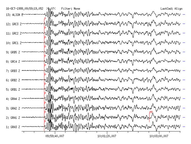
**Figure 9a** Broadband vertical-component seismograms recorded at 12 GRF-array stations. Traces are sorted according to increasing distance ( $D = 83.6^{\circ}$  to GRA3 and 84.4° to GRC3), shifted in time and aligned for P onsets. The coherent phases P and PP are marked, however some more onsets appear ahead of PP.
