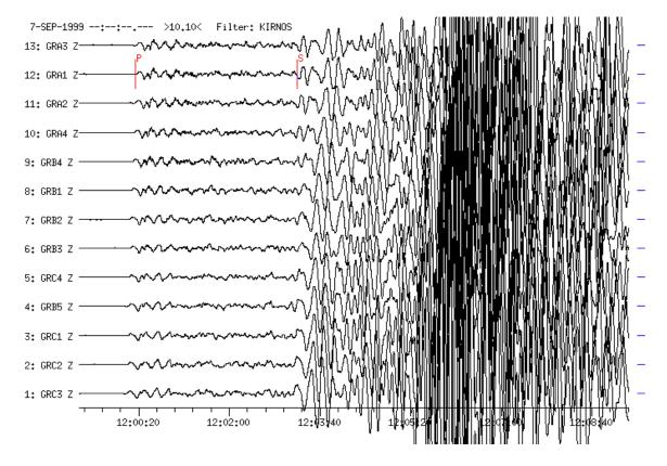
**Figure 1c** KIRNOS-filtered seismograms of vertical-component records at the GRF-array stations sorted according to increasing epicentral distance ( $D = 13.8^{\circ}$  to GRC3 and 14.6° to GRA3). Note the variability of waveforms within the S-wave group.
