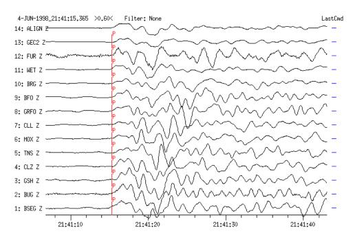
**Figure 4a** Broadband vertical-component seismograms recorded at 13 GRSN stations. Traces are sorted according to increasing epicentral distance ( $D = 18.9^{\circ}$  to BSEG and 24.2° to GEC2), shifted in time and aligned for better signal comparison. All signals are incoherent and influenced by upper mantle discontinuities.
