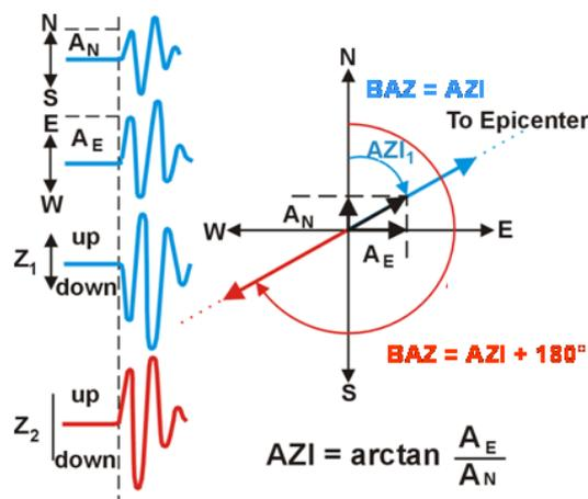
**Figure 1** Synthetic example of P-wave first motions in 3-component records (left) from which the azimuth AZI (clockwise from north towards the direction of wave-propagation), respectively the backazimuth BAZ (clockwise from north towards the direction of the source as seen from the station) can be calculated.
