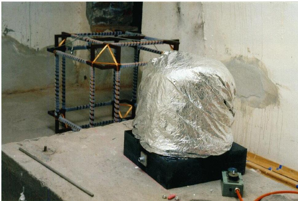
**Figure 5** The whole installation is wrapped with a reflective foil which can be obtained as a part of first-aid kits. The reflective foil reduces radiative and convective heat transport and therefore is part of the thermal insulation. Again it is recommended to extend the foil over the gabbro plate down to the surface of the pier. Ensure that no air-draft can pass underneath the foil. Tape it to the pier or put some heavy items on its edges.
